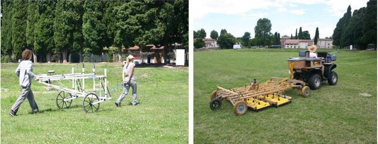
Fig. 19. Magnetic (L) and GPR survey (R) by the Ghent University team (photograph Frank Vermeulen).
